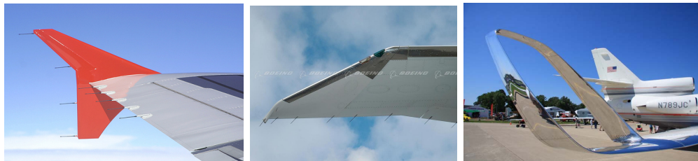
(d) Wingtip fence. By: http://www.flickrriver.com/photos/tags/wingtipfence/interesting/ (e) Raked wingtip. By: http://www.boeingimages.com/ (f) Spiroid tipped wing. By: https://es.pinterest.com/ahmadh_89/aircraft-winglet-design/
