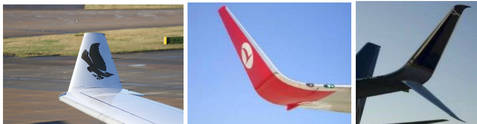
(a) Winglet. By: https://www.flickr.com/photos/mals_r/8471335777 (b) Blended winglet. By: http://flitetest.com/articles/why-do-planes-have-winglets (c) Up-down winglet. By: http://flitetest.com/articles/why-do-planes-have-winglets
