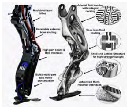
Figure 10: Boston Dynamics' Atlas 2016 Leg Detail
