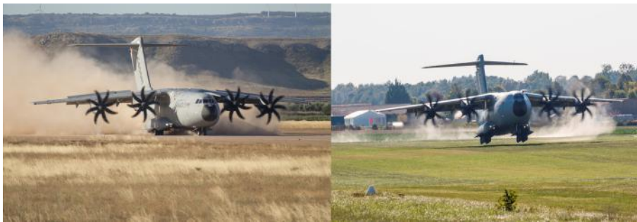
Figure 1.15 A400M on gravel (left) and grass (right) runway tests
