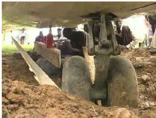
Figure 1.13 Limiting case: partially buried landing gear
