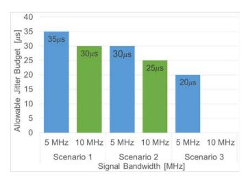
Fig. 6. Fronthaul Allowable Jitter Budget with a latency close to the Limit in Scenario 1, Scenario 2 and Scenario 3
