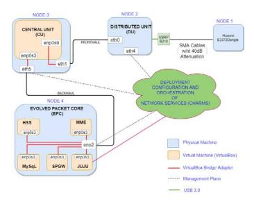
Fig. 4. Scenario 3: virtualization of CU and EPC
