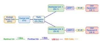
Fig. 3. Scenario 2: Multiple DUs and Multiple UEs
