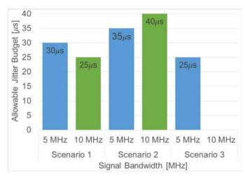
Fig. 7. Fronthaul Allowable Jitter Budget with a latency from the Limit in Scenario 1, Scenario 2 and Scenario 3
