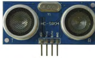
Figure 6.3: Chosen ultrasonic rangefinder: HC-SR04. Source: arduinolearning.com
