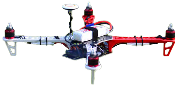
Figure 6.15: Default F450 configuration. Source: rcgroups.com
