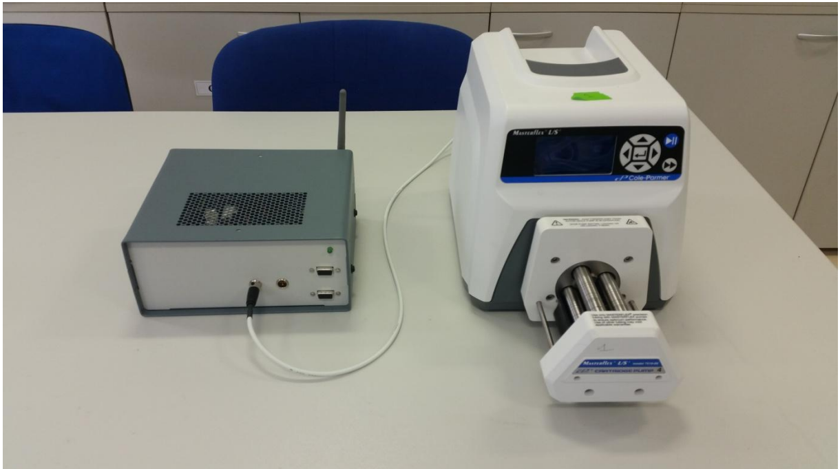
21 Modular box I connected to one of the Masterflex L/S 7523 pumps
