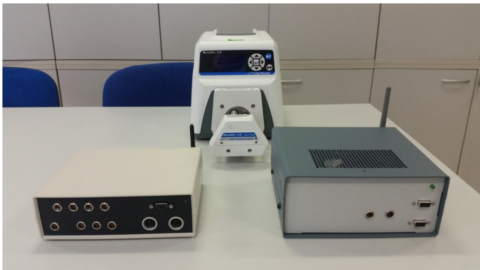
24 (Left) Finished modular box 2, with the top inputs for thermometers, the bottom ones from left to right: level and weights. To the right, the RS-232 connector for the CDI and below the connectors for the thermostats.
