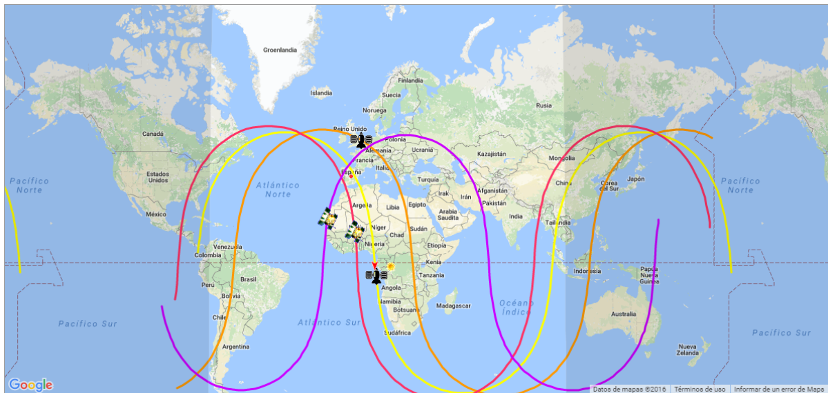
Figure 6.5: GPS Satellite Trajectory. (Source: N2YO.com)
