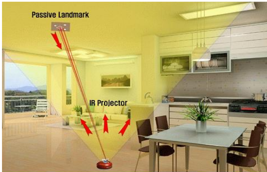
An illustration showing how StarGazer™ works.
