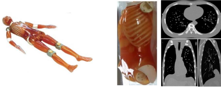
Figure 4.8 (Left) Whole PBU-50 anthropomorphic phantom, (middle) thorax of PBU-50 phantom and (right) axial, coronal and sagittal views of the CT volume
