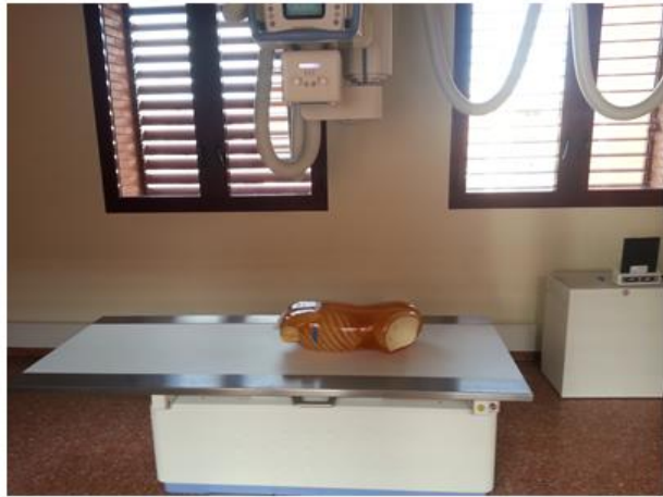
Figure 4.18 (Left) Diagram showing implemented tomosynthesis protocol (Right) Middle autoposition (number 11) of the tomosynthesis protocol in the X-ray room
