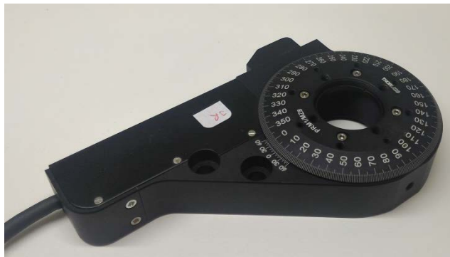
Image 31. Motor whose rotation is responsible for the selection of the LED that is going to be used at each moment
