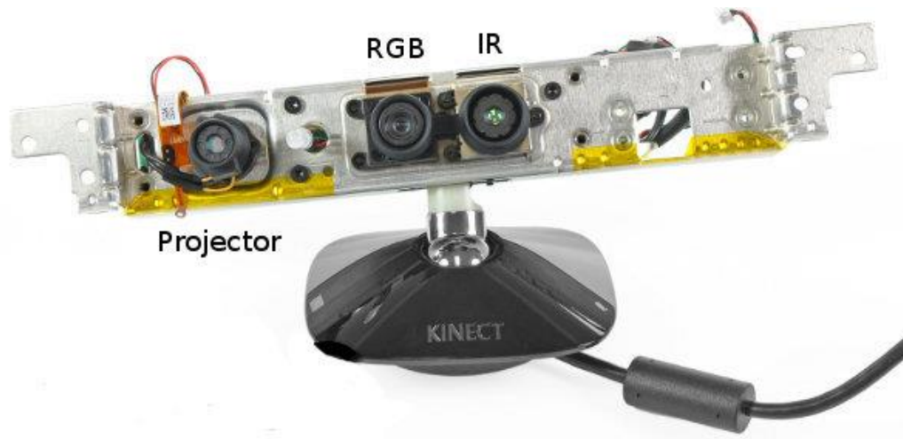
Figura 13. Interior de la Kinect.
