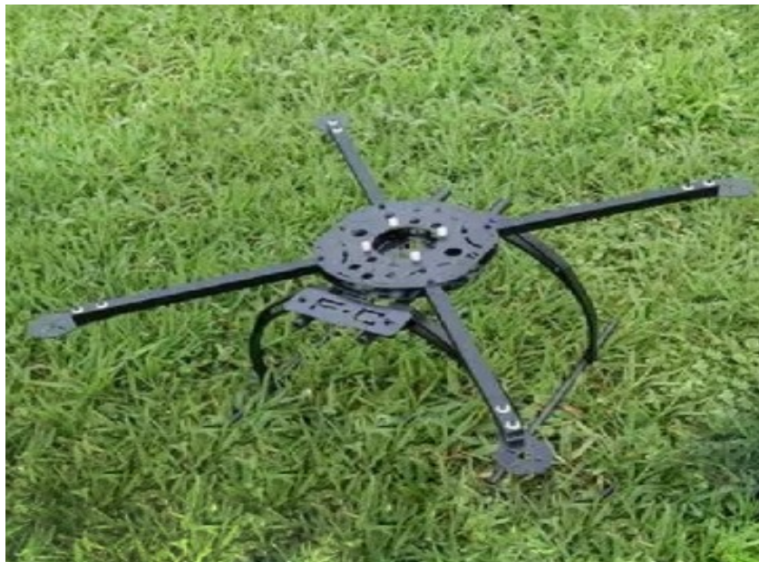
Figure 3-5: FC X580 580MM folding quadcopter frame carbon and fiber landing gear.
