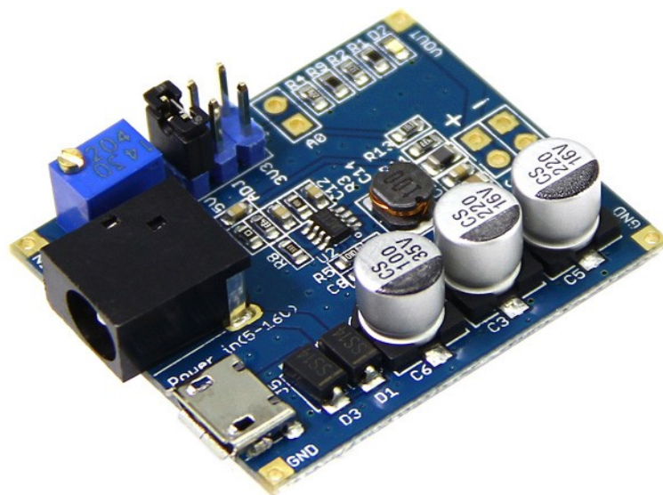
Figure 3-50: Adjustable DC/DC Power Converter
