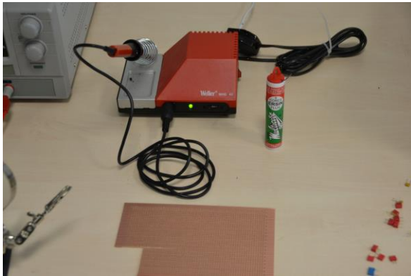
Welder + Sn + Cu connection board
