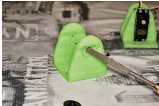
(b) If needed, file the hole until the servo horn fits tightly on it.
