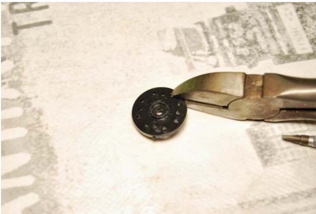
(c) With the help of some cutting pliers, cut the horn with the shape of the corresponding hole in the printed part.
