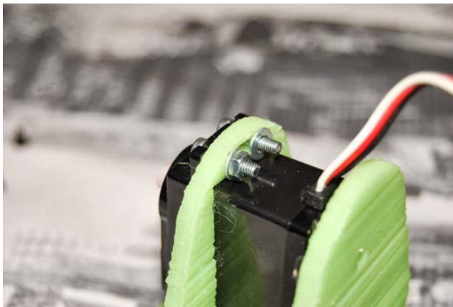
(c) Fix the servo to the module using the screws, nuts and washers for the top holes.
