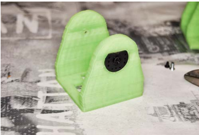
(e) Insert the horn in the corresponding hole of the upper part.
