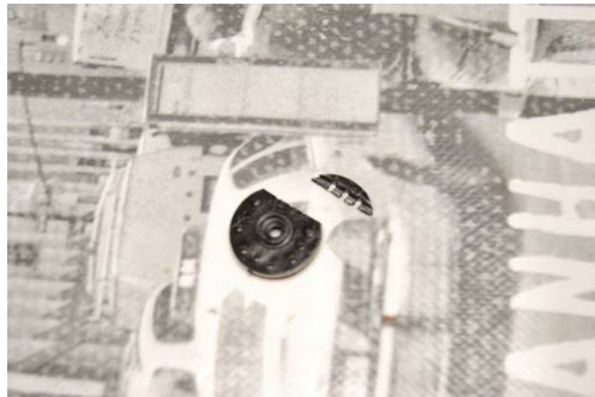
(d) After the cut, the servo horn should look like this.
