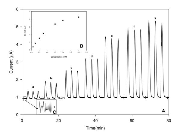
Given the device configuration and the hydrodynamic parameters used, it was possible to obtain a sampling throughput of 38 samples hour<sup>-1</sup>.
