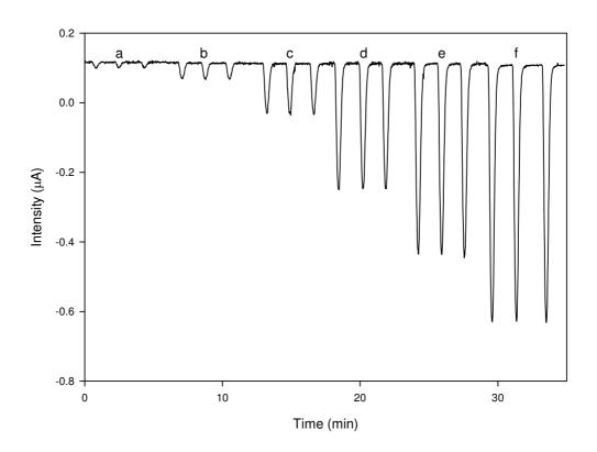
The linear regression at its linear zone was founded to be  $I = 3.7E^{-08}(\pm 0.1E^{-08}) - 1.1E^{-07}(\pm 0.004 E^{-07}) \cdot [C]$  (n=3; 95% confidence; r<sup>2</sup>>0.998). Where: I is the current flowing in the cell and [C] the analyte concentration. For an intermediate concentration (3.5mM), the RSD obtained was 1.93% (n= 15; 95% confidence).
