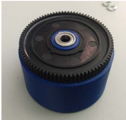
Fig. 53 Finished wheel system. Notice the ball bearing in the center, the wheel itself (blue) and the spur gear (black).
