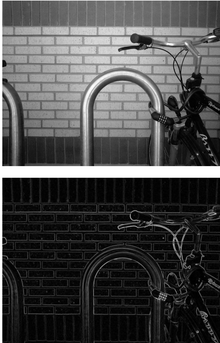
Fig. 11. Comparison of the original image and the result after applying the Sobel operator [36][37].
