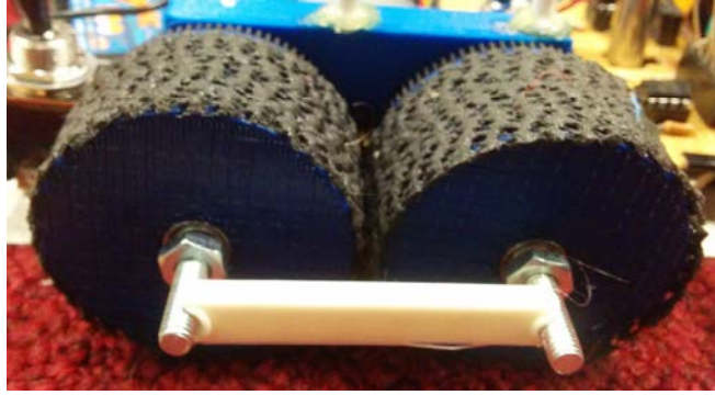
Fig. 46 Wheel separator to correct the alignment of the wheel axis.
