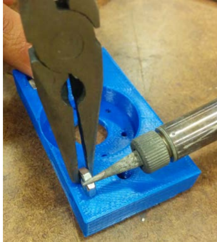
Fig. 29 Inserting the nuts into the motor mount using the heat from the soldering iron.
