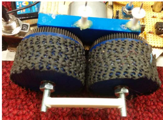
Fig. 55 Mounted transmission system. Notice the separator and the anti-slip "homemade" tires.
