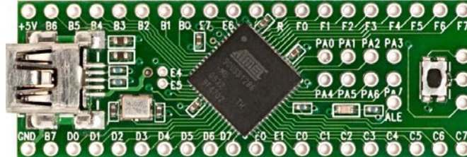
Fig. 7. Teensy 2.0++ has more than 40 I/O pins while the Arduino nano only has 28 [20][21].
