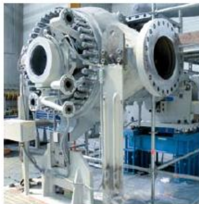
SST-700 HP Turbine module in the German workshop.
