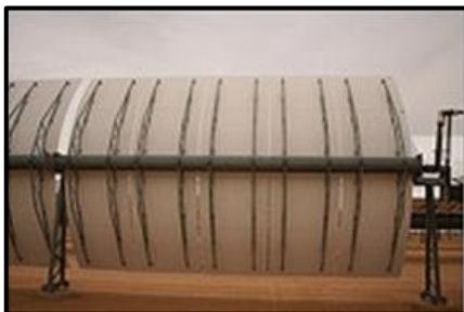
Figura 43. Estructura del colector LS-2 (National Renewable Energy Laboratory (NREL)).
