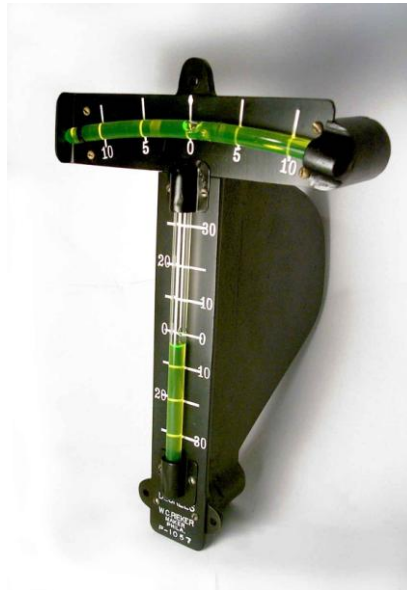
Illustration 3. Spirit of Saint Louis bubble inclinometer
