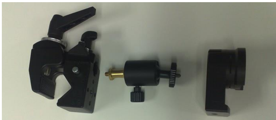
Figure 14 From left to right: camera clamp, camera-to-clamp connector and camera.
