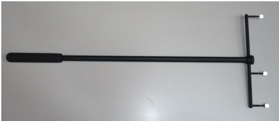
Figure 16 OptiWand, a tool used to calibrate the cameras.
