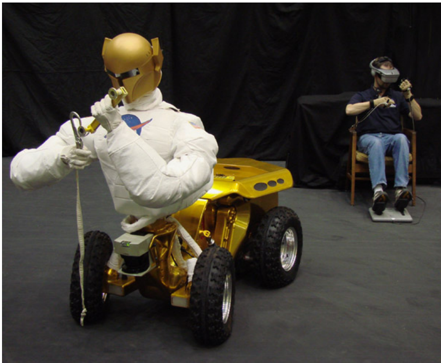
Figure 3: Operator controlling the Robonaut coupled to the Centaur
