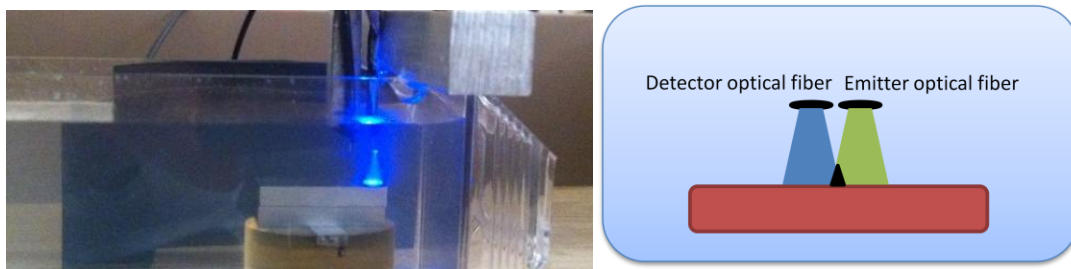
Figure 6.1 Backward configuration of the system. Real system (left) and ideal scheme (right).
