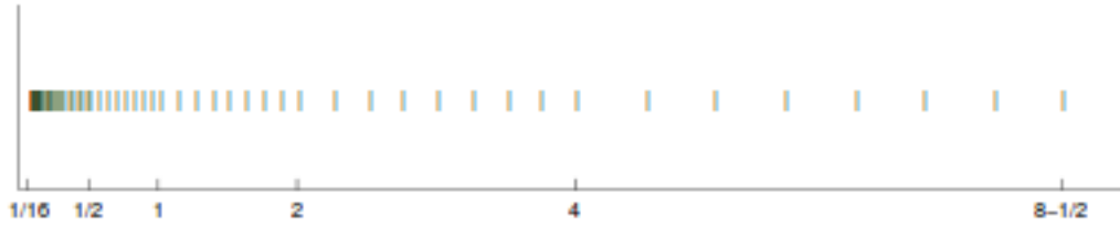
Figure 1: Floating point arithmetic representation with t = 3, emax = 3, emin = -4 , from the program floatgui of [26].
