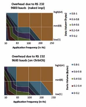
Fig. 10. Benchmark results. Overhead (16 MHz-ATmega328–2.5 Ghz Real-time Java stack via a 9600 RS-232 link). Application maximum frequencies ranging from 10 Hz to 0,25 kHz
