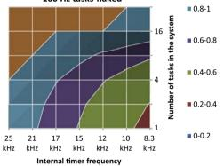
Fig. 4. Benchmark results. Scheduling System Overhead (16 MHz-ATmega328) with naked implementation.
