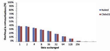
Fig. 9. Performance results. Overhead (16 MHz-ATmega328-2.5 Ghz Real-time Java stack via a 9600 RS-232 link) due to end points (CPU and runtimes).
