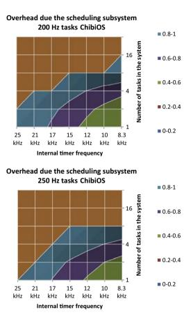
Fig. 6. Benchmark results. Scheduling System Overhead (16 MHz-ATmega328) with naked implementation.
