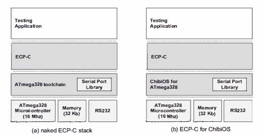
Fig. 2. The two ECP-C implementations: naked ATmega328 and ChibiOS for ATmega328.
