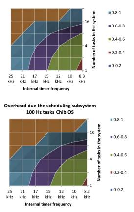
Fig. 5. Benchmark results. Scheduling System Overhead (16 MHz-ATmega328) with a ChibiOS implementation.
