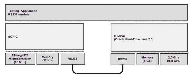
Fig. 8. Stack used to benchmark the RS-232 interface when it is used to communicate a Java application with an ECP-C application.
