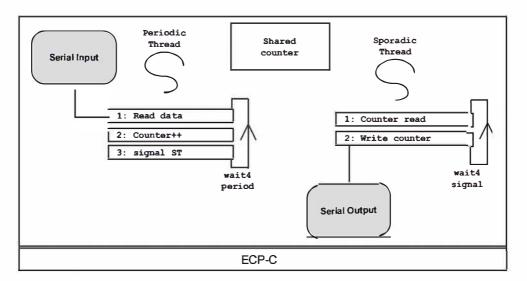
Fig. 1. ECP-C example application with two threads sharing information.
