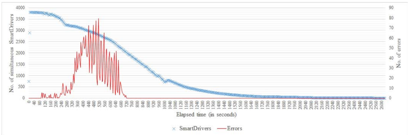
Fig. 11. Ztreamy using server type 1 and errors occurred during the simulation.
