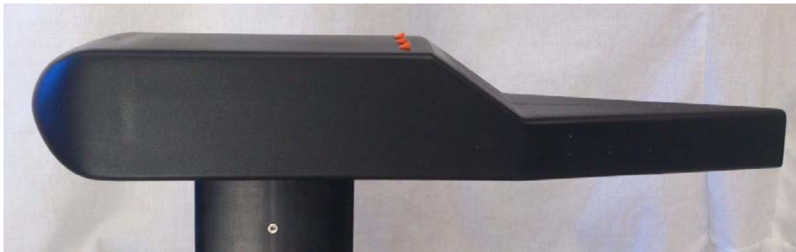
Figure 4.13 Helicopter mock-up (turned upside-down) with the Vortex Generators employed sitting on top (orange color).
