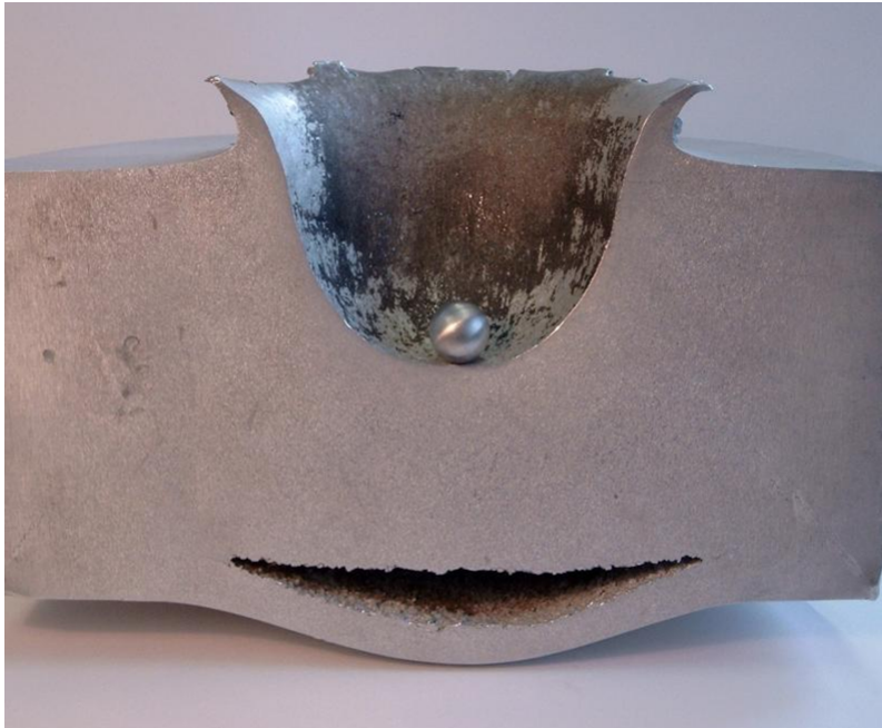
Figure 1.5: Effects of a hyper-velocity impact, (Photo provided by ESA)
