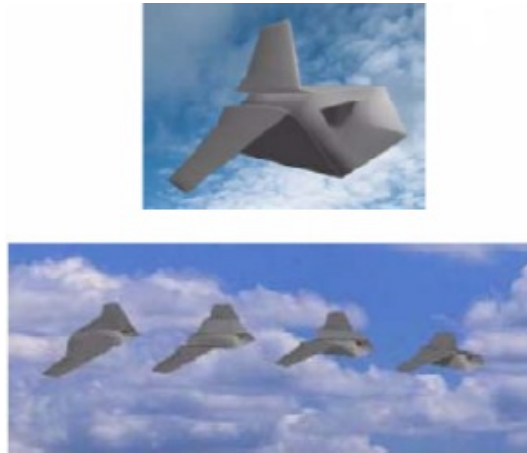
Figure 1.4: Morphing Wings in the Lockheed Martin Unmanned Air Vehicle (UAV) Concept [19]
