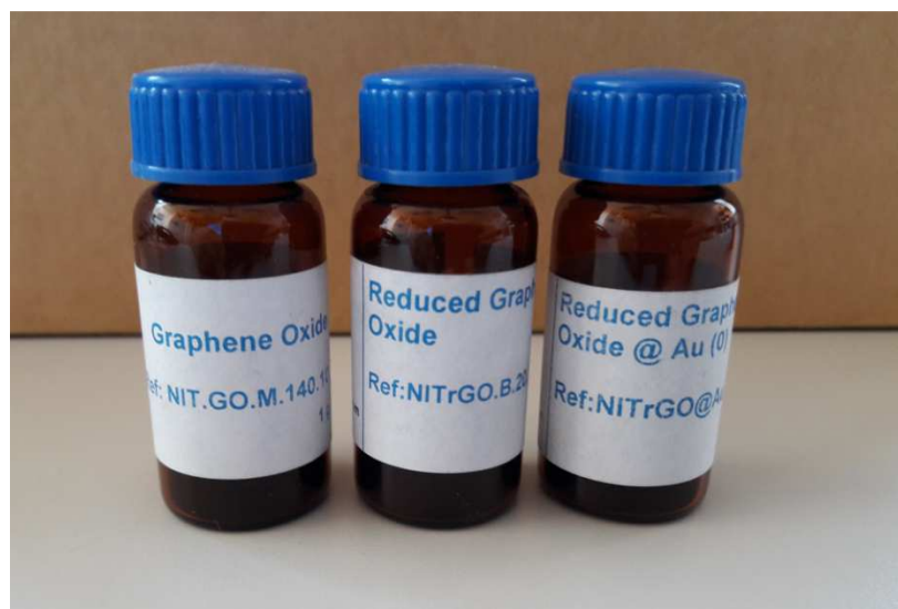
Figure 3.7. Samples of GO, rGO, and rGO@Au used in our optoacoustic experiments (concentration of 50 \mu\text{g/ml} ).
