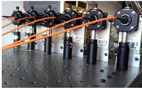
Figure 4.6. The beam emitted by the HPDLs is coupled side-by-side into optical fibers with variable core diameter by collimating and focusing lenses in a xyz translator mount.
