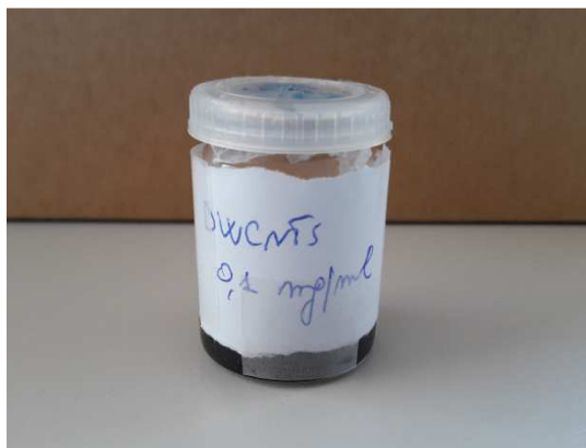
Figure 3.2. Samples of DWCNTs used in our optoacoustic experiments (concentration of 0.1 mg/ml in distilled water).
