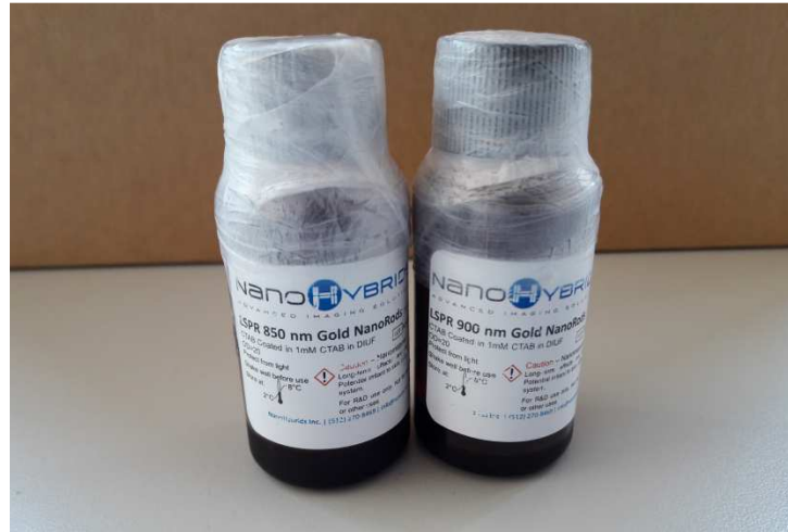
Figure 3.10. Samples of gold nanorods used in our optoacoustic experiments (concentration of 0.8 and 0.9 mg/ml, respectively).
