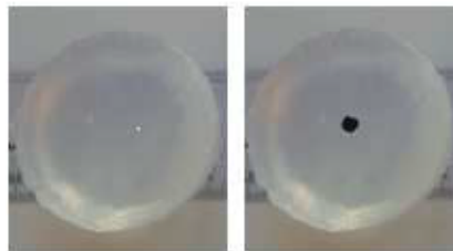
Figure 4.10. A tissue-like cylindrical phantom composed of 10% of agar and 90% of neutral gelatin, diluted with distilled water: a) directly after preparation, and b) with a 2 mm × 30 mm (diameter × height) ink-filled inclusion.
