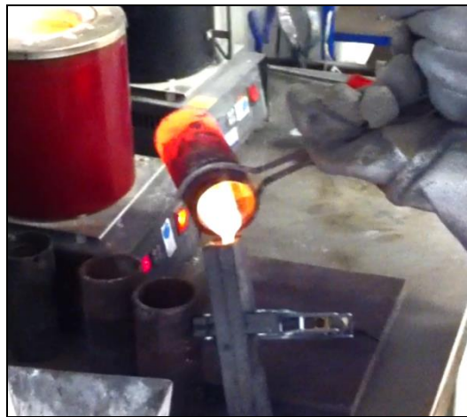
Figure 6: Melt being poured into the mild steel die
