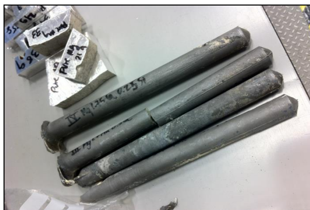
Figure 7: Master alloys (top left corner) and gravity cast Mg alloy rods
