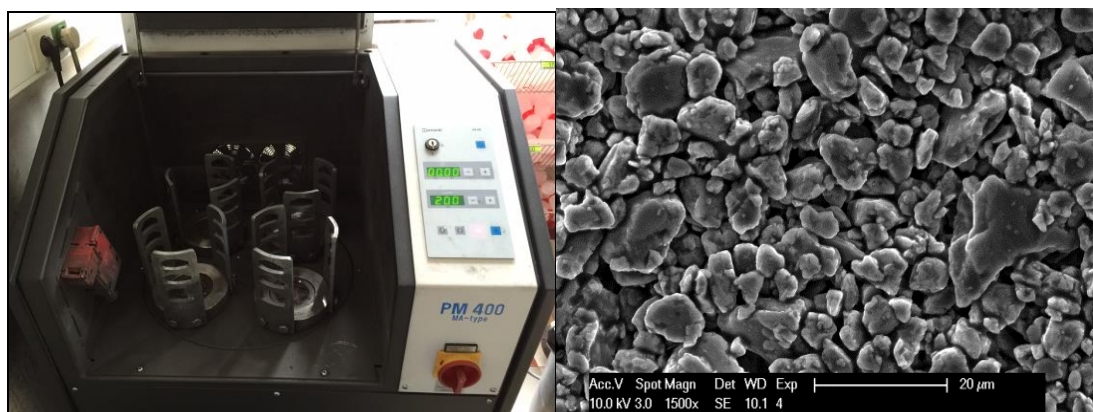
Figure 14: Opened PM 400 MA-type planetary mill (left) & Powder product (right)
