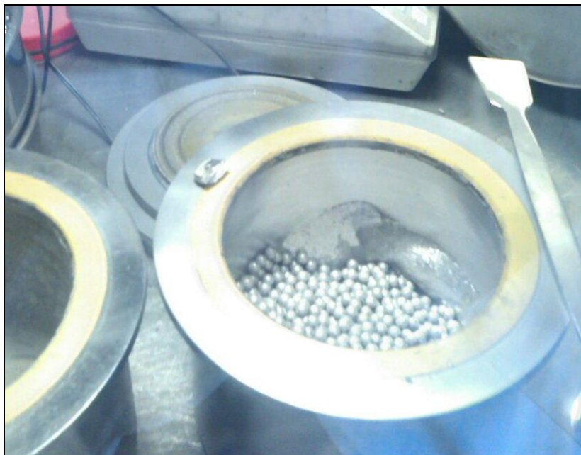
Figure 16: Material stuck to milling media and vessel wall
