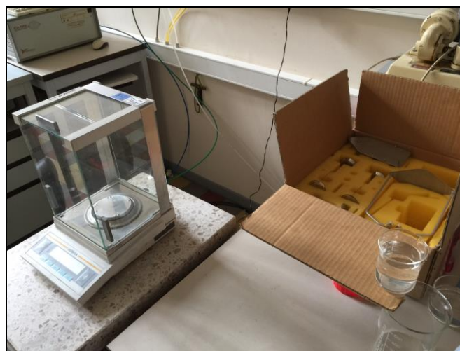
Figure 19: Archimedes density measurement kit
