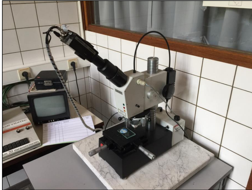
Figure 12: Durimet microhardness tester
