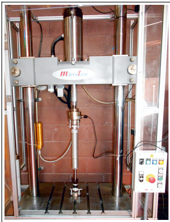
Figure 11. S46WRICI Öhlins damper installed on a damper test machine.
