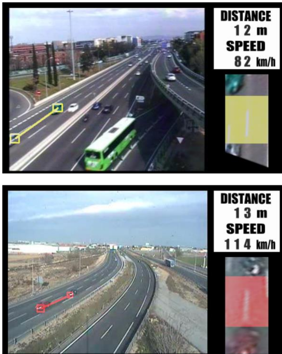
Figure 50. Output visualization examples; yellow marks moderate infraction, red marks severe infraction.
