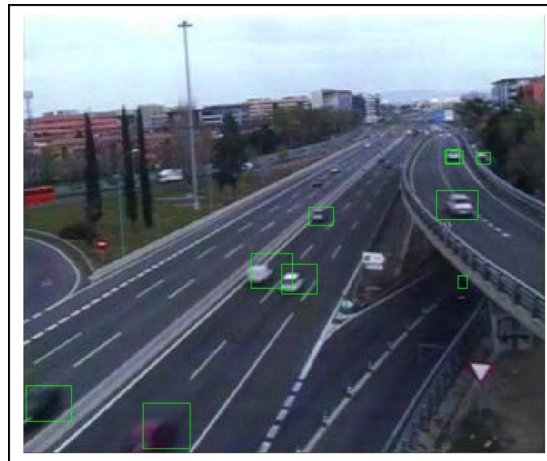
Figure 43. Vehicle trajectory trackers displayed as bounding boxes for a certain frame. Bounding boxes are simple and approximated representations of vehicles shapes and locations
