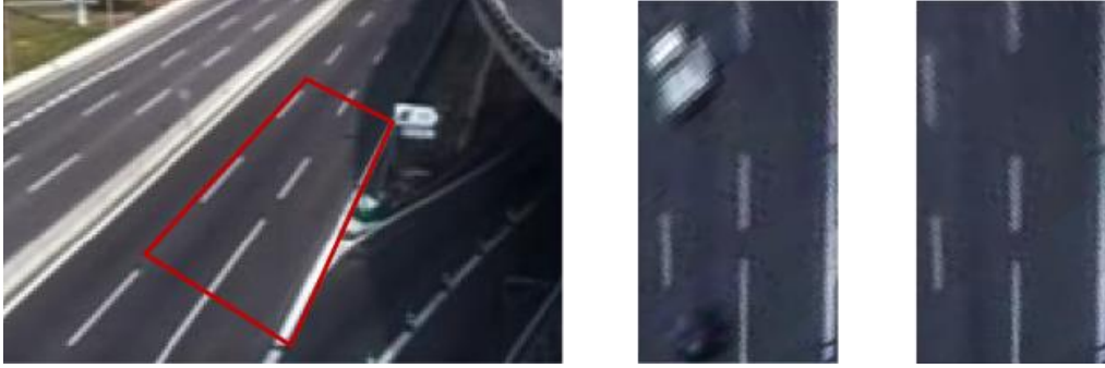
Figure 41. Detected DA in a scene (left). For a given frame in the video, normalized top-view of the DA (middle) and the background DA (right).
