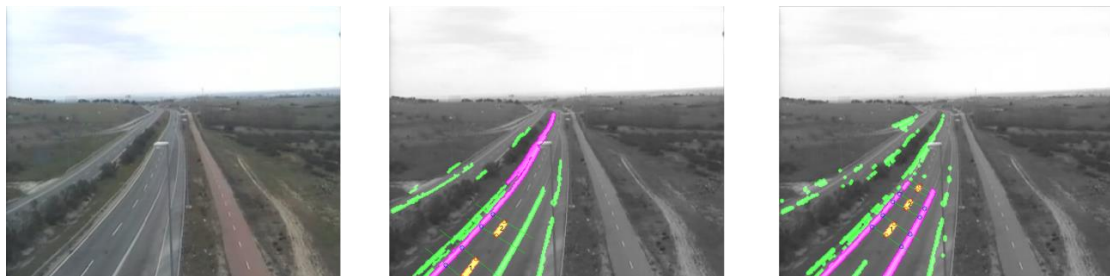
Figure 63. Performance of the automatic (middle) and the semi-automatic (right) method for camera location 7.
