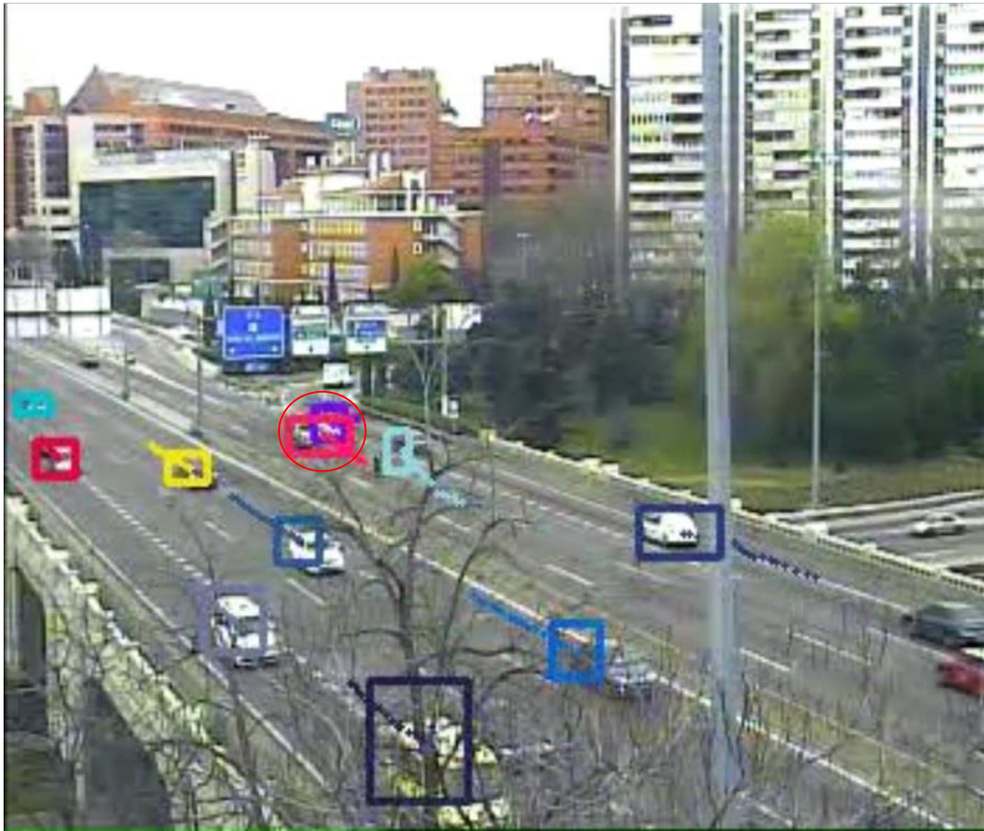
Fig. 1.2: high traffic situation in which the tracker “jumps” from a motorbike to a car.
