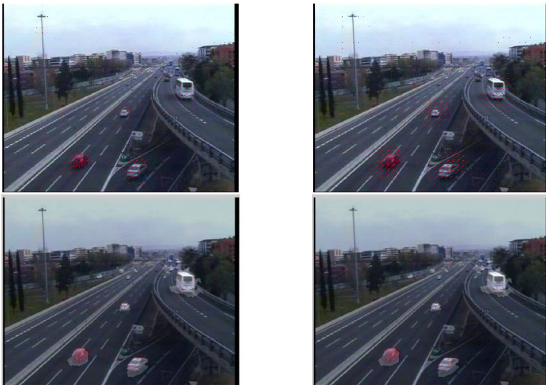
Fig. I.2: resultant vectors from motion estimation with L&K algorithm. Left, r=5 , Right, r=15 . Above, without applying foreground mask. Below, applying foreground mask.
