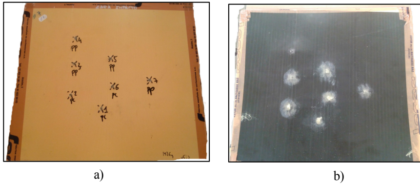
Figure 3. Final stage of the STANAG 2920 tests for seven shots. a) Front and b) back sides.
