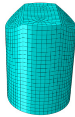
Figure 1. Numerical model of Fragment Simulating Projectile (FSP).
