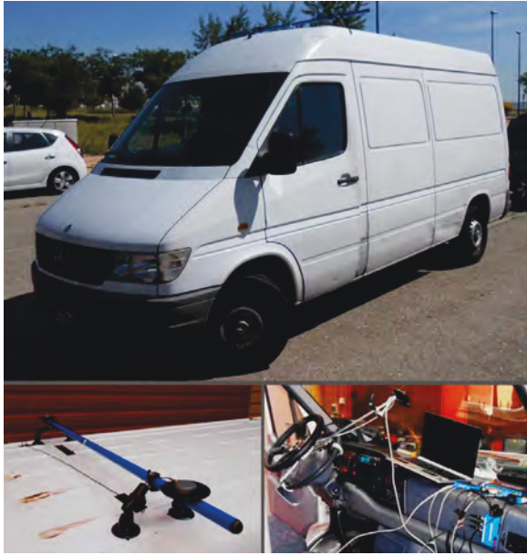
Fig. 3. Experimental setup on a test vehicle (Mercedes Sprinter).
