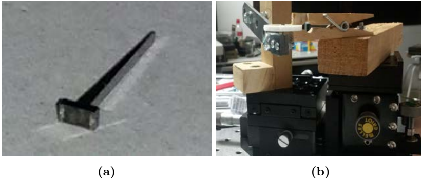
Figure 3.8: Device assembly: The AE is glued to the DRW antenna: photo (a) shows a Log-periodic AE glued to a H-plane tapered DRW antenna. Secondly, it is centered and aligned to the axis of a 1 inch diameter 3 mm thick foam disc. Two micropositioners with custom holders are used in this step.
