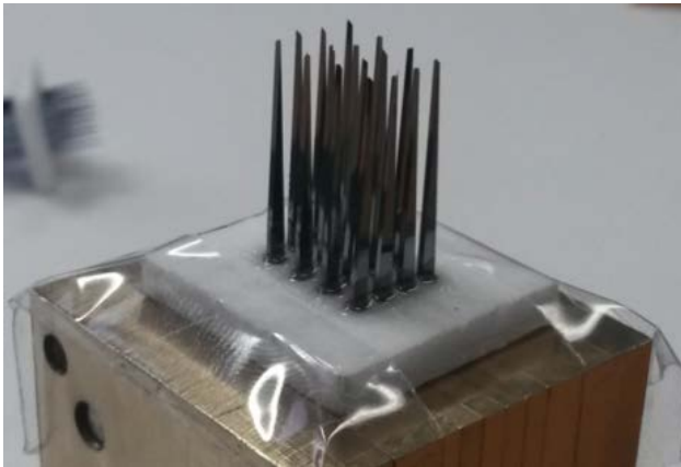
Figure 5.5: DRW antennas array fully assembled.
