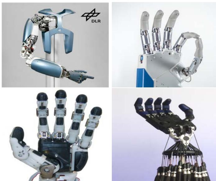
Figure 1.1: Examples of anthropomorphic robotic hands. Top-left: DLR hand-arm system. Top-right: Azzurra hand. Bottom-left: Elu2 hand by Elumotion. Bottom-right: Shadow hand.
