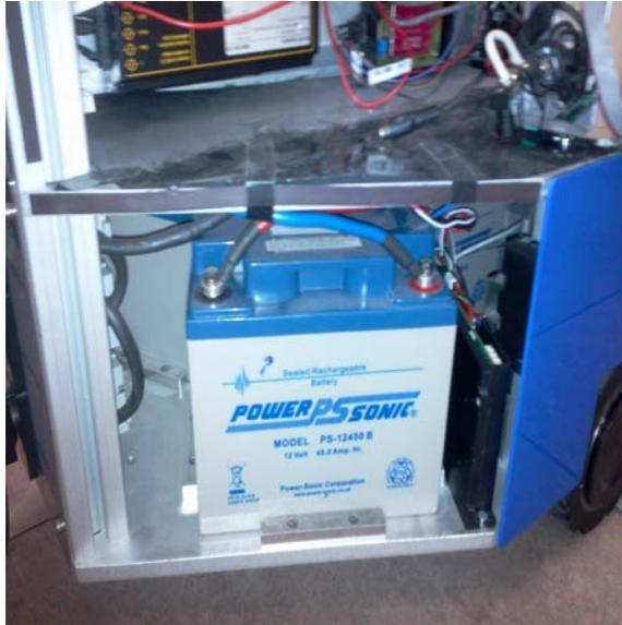
Figure B.3: Power supply system.
