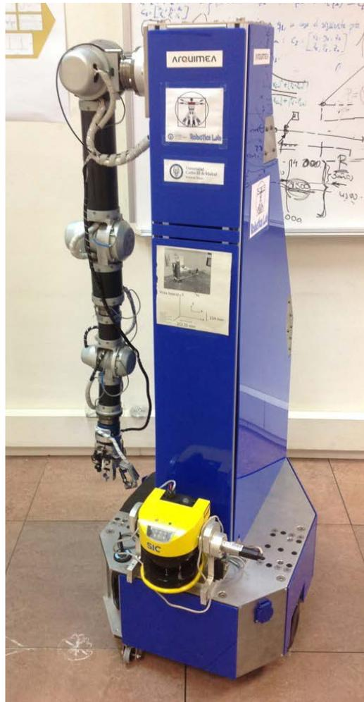
Figure B.1: ManfredV2, mobile manipulator with robotic arm.
