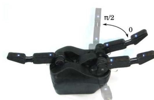
Figure B.16: Angular limits of the preshape joint of Reflex TakkTile Hand.
