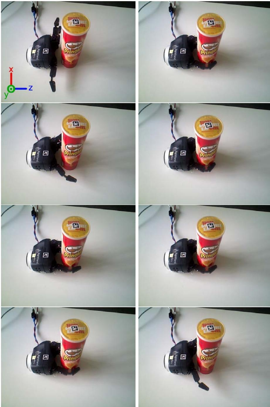
Figure 4.11: Scenario 1, a Pringles can grasped while the hand lies on the surface of the table.
