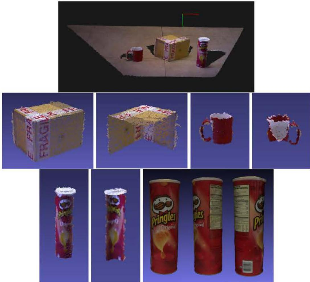
Figure 3.2: At the top, a scene with several objects lying on a surface. Below, the cloud of the non-recognised objects extracted from the scene after Euclidean segmentation is applied. In the third row, besides the cloud of the object, several views of the corresponding 3D model of a recognised object can be seen.
