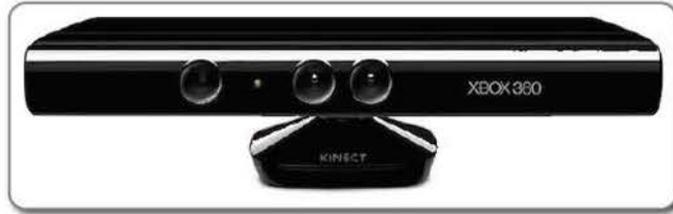
Figure B.10: Time-of-flight camera: Kinect.
