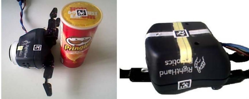
Figure 4.8: On the left, the robotic hand lies on the table ready to perform a grasp. On the right, the tags needed to locate the reference frame for the pose estimation of the base of the hand.
