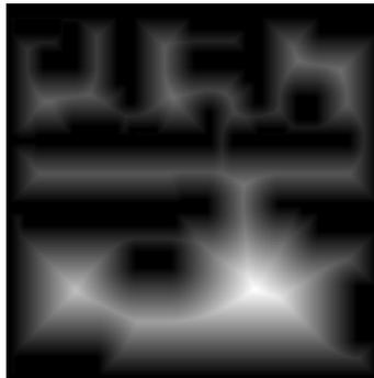
Figure 2.3: Example of a *slowness map*, result of computing the FMM to an occupancy map and considering all the obstacles as sources of a wave.
