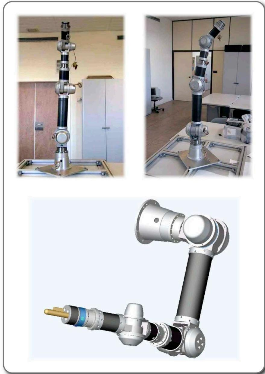
Figure B.4: LWR-UC3M-1(robotic arm).
