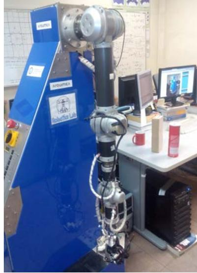
Figure 3.25: Scene for grasp testing. Objects are positioned on the table for the robot to grasp them.
