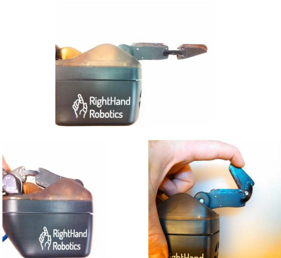
Figure B.15: Angular limits of the joints of the fingers of Reflex TakkTile Hand.
