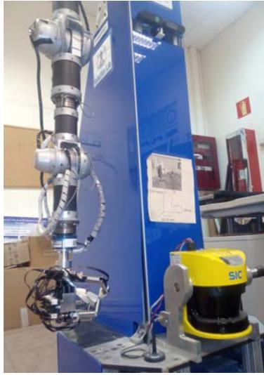
Figure 3.17: Starting configuration of the hand to avoid a collision with the base.
