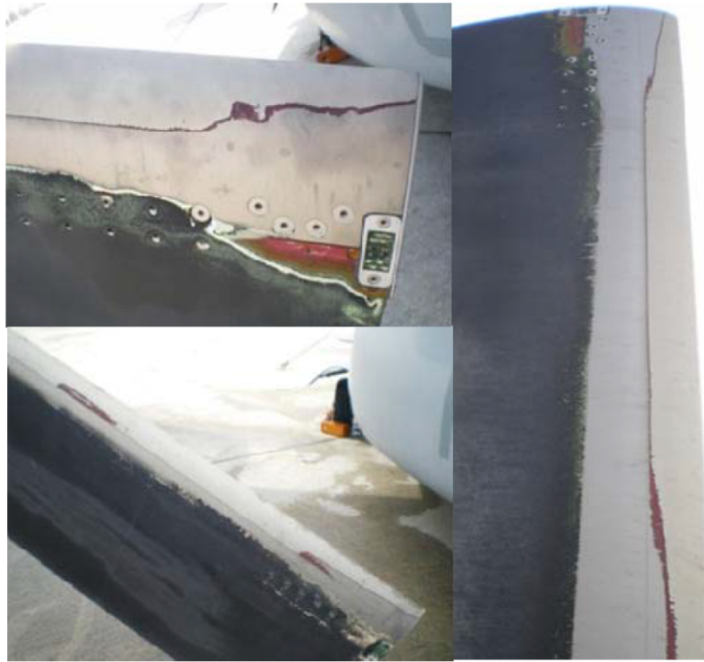
Figure 32: Erosion from field observations of V-22 Osprey [32].
