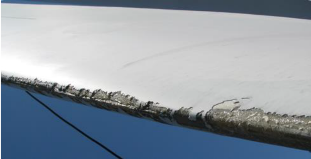
Figure 7: Example of leading edge erosion [16].
