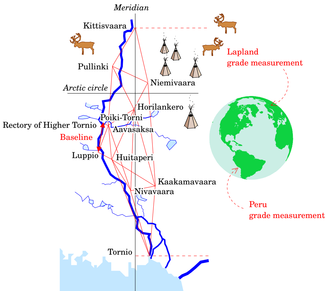
FIGURE 1.7. The grade measurement project of the French Academy of Sciences: the Lapland grade measurement network.
