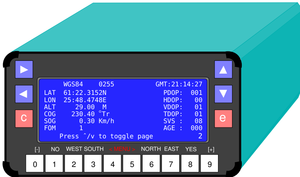
FIGURE 12.10. Control panel of the Ashtech Z-12.
