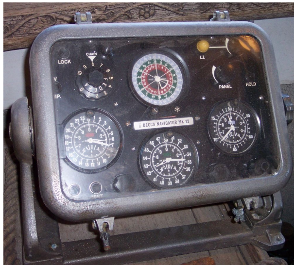
FIGURE 12.2. A Decca receiver. Wikimedia Commons, Decca Navigator Mk 12.
