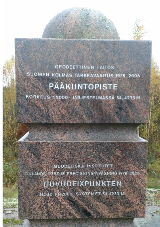
FIGURE 3.16. Fundamental benchmark PP2000 of the N2000 height datum at the Metsähovi research station. Established by the Finnish Geospatial Research Institute (FGI) of the National Land Survey of Finland.
