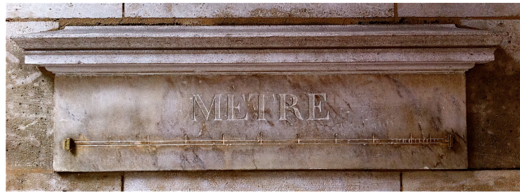
FIGURE 2.1. A public standard metre in Paris. Wikimedia Commons, Standard metre in Paris.
