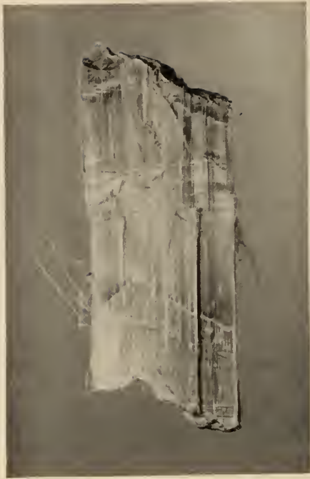
ASBESTOS ( left ) is a variety of serpentine, a hydrous magnesium silicate consisting of white, gray, or green fibers which are easily separated and can be spun or filtered to make non-combustible fabrics
