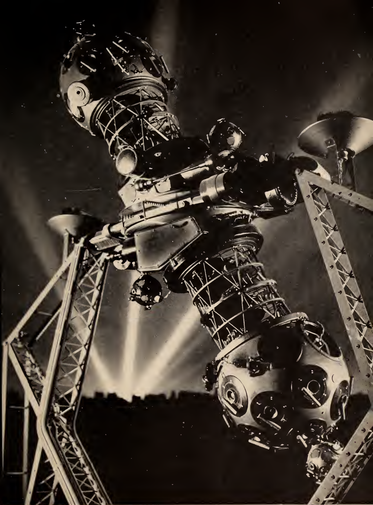
THE GREAT PROJECTION INSTRUMENT IN THE HAYDEN PLANETARIUM. This is the principal feature of the Planetarium building. Through its means the illusion of the heavens with the fixed stars and planets, following their apparent paths through the sky, is thrown upon a dome-shaped ceiling
