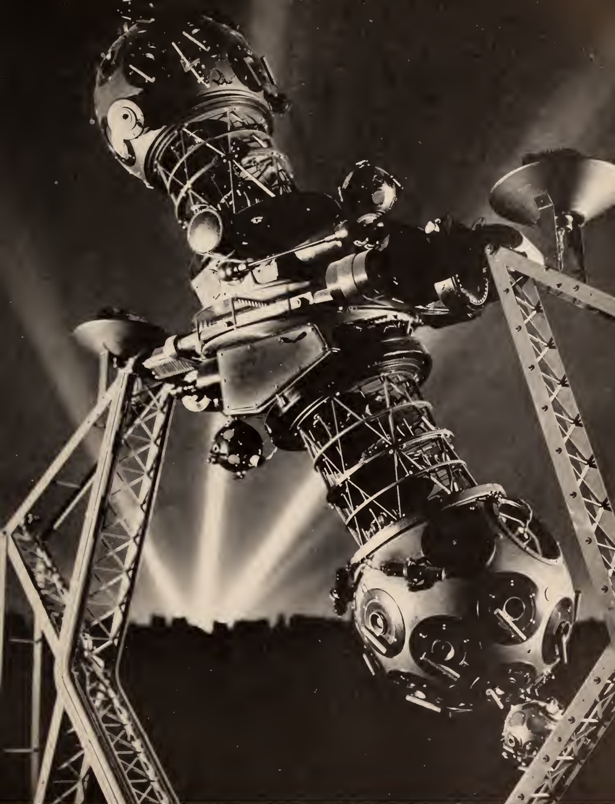
THE GREAT PROJECTION INSTRUMENT IN THE HAYDEN PLANETARIUM. This is the principal feature of the Planetarium building. Through its means the illusion of the heavens with the fixed stars and planets, following their apparent paths through the sky, is thrown upon a dome-shaped ceiling
