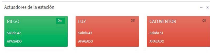
Fig. 9. Actuator control from the webpage
