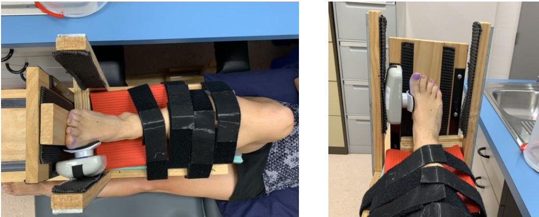
Figure 8-1 Test position for plantar flexion-inversion force with fixed hand held dynamometer
