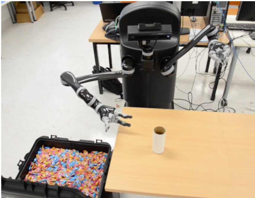
Figure 4.2: The problem scenario for the CandyScooper problem. A MOVO mobile manipulator equipped with a 6DOFs Jaco arm with KG3 gripper must pick-up a cup located on a table in front of the robot, use the cup to scoop candy from a candy box located next to the table, and put the cup back on the table.
