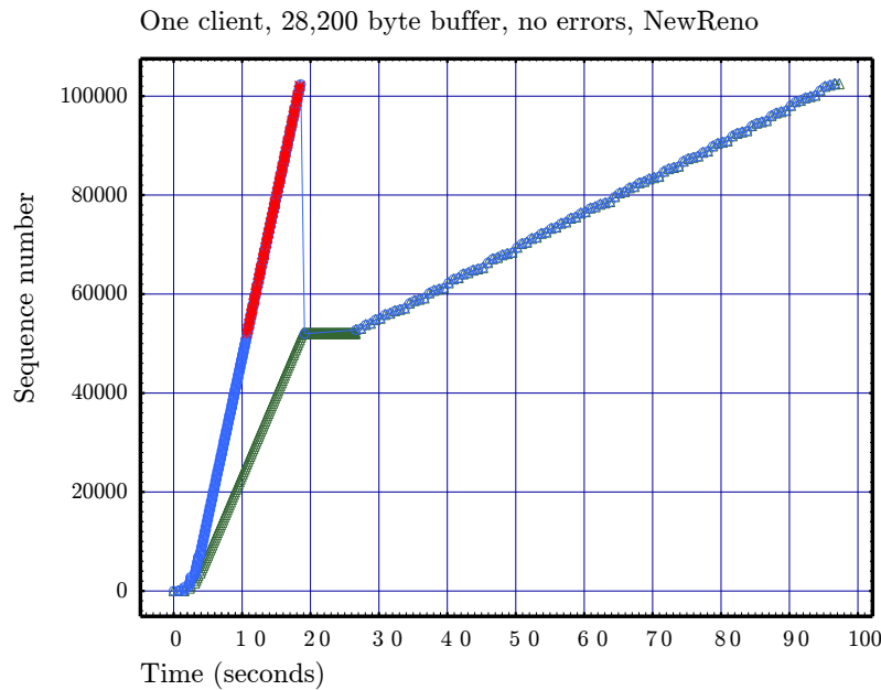
Figure 16: Time-sequence graph for a single TCP New Reno flow. Sent segments are blue, received acknowledgements green, and dropped segments red. Image shows overshooting in Slow Start. Most data cannot fit in the buffer and is dropped. Resending is slow as only one segment can be sent per ACK.
