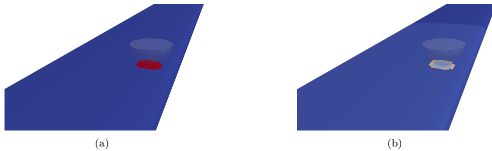
FIGURE 6.16: (a) Non-linearities in the macro-scale (in red) and the elements that remained in the linear region (in blue). (b) Computational cost distribution at the macro-scale.
