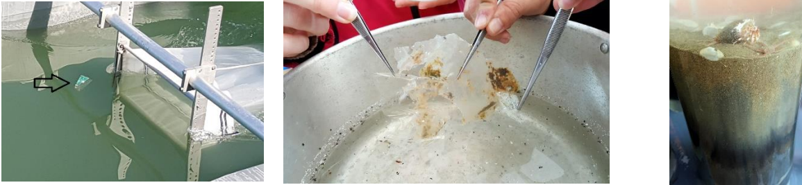
Figure 2. (L-R) Macroplastic object passing outside the catamaran trawl opening (station 7), large plastic fragments collected in the catamaran trawl (note also the abundant white plastic foam particles on the sides of the aluminum sampling container; station 7), sandy sediment core near the Thames estuary with hermit crab and brittle star (station 8).
