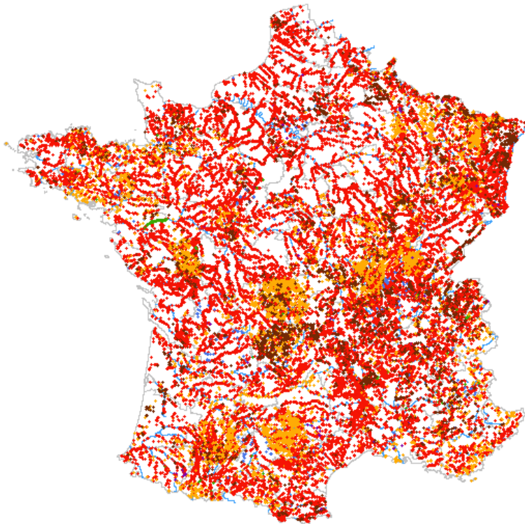
Figure 13: ROE map of obstacles in river systems of France. Each dot represents an obstacle, color gradient represents the height (towards red = higher obstacle)
