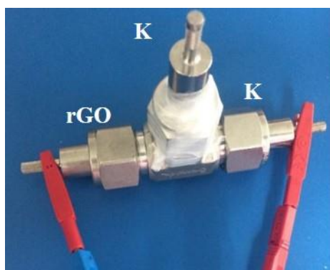
Figure S7. Three electrodes setup used to run impedance tests.
