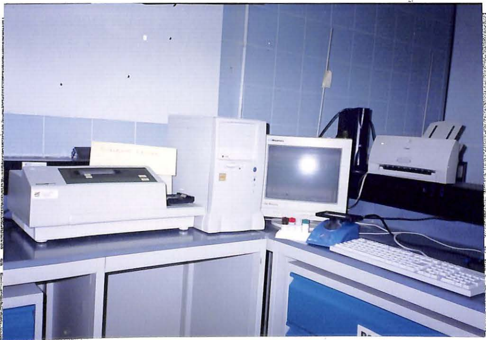
3.1.2 Photograph 2 : The photograph shows the "microplate reader" and the computer involved in ( ELISA ) method .
