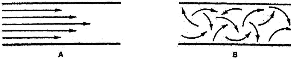
Fig. 5 : Airflow patterns. A, Laminar flow. B, Turbulent flow.
